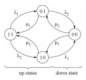
State diagram of a Markov Process representing an AND gate with two basic events. The MP is down when all base MPs are down.
