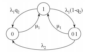
State diagram of an MP representing a dynamic variant of the AND gate. The MP is down while being in state 0.
