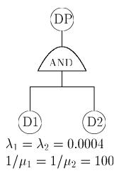
Fault tree representation of the Detector Package consisting of two identical detectors connected in parallell.
