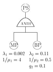
Fault tree representation of the Power Supply. Its components are the Main Power (MP) and the Back-up Power (BP) sub-systems.
