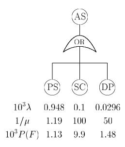
The complete Alarm System consist of a Power Supply, a Supervising Computer and a Detector Package.
