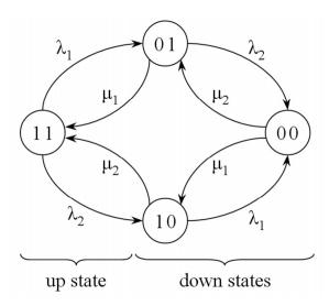
State diagram of a Markov Process representing an OR gate with two basic events. The MP is down if at least one base MP is down.
