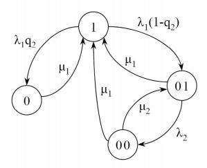
State diagram of an MP representing a 2nd dynamic variant of the AND gate. The MP is down while being in state 0 or 00.
