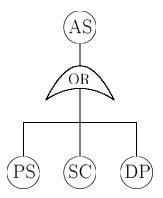
An Alarm System that consist of a Power Supply, a Supervisong Computer and a Detector Package.
