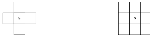
Figure 4.2: Two often used neighbourhood systems: to the left the site s has four neighbours and to the right it has eight neighbours.
