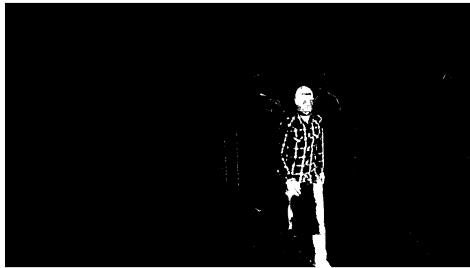
(b) Foreground pixels of frame after modelling the background with Mixture of Gaussians.
