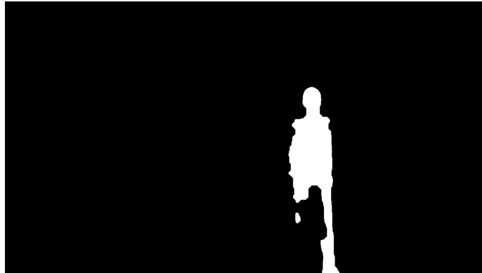
(c) Foreground pixels after noise removal with a median filter and applying opening and closing morphological operations.
