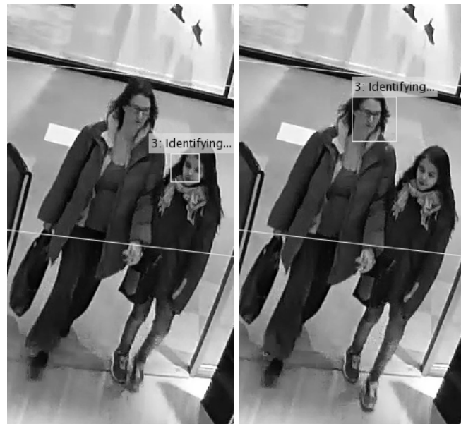
(a) Predicted location of individuals face. (b) New detection gets assigned to the same existing track.
