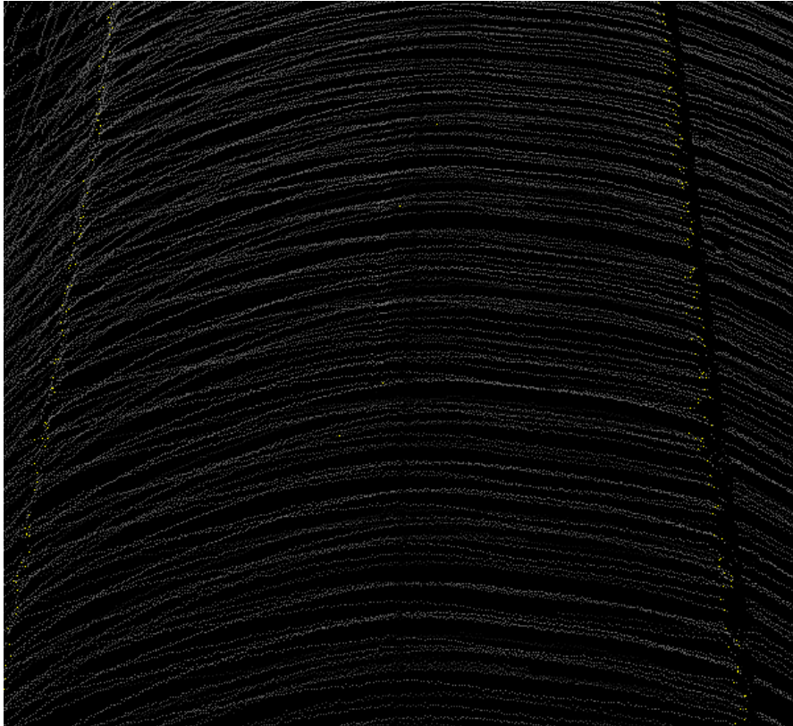
Figure 3.3: This figure represents a typical example of how curbs are found using Algorithm 5. Yellow points are the estimated road edges.
