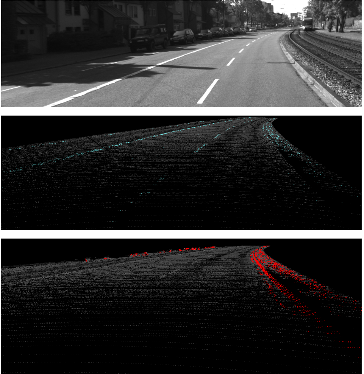
Figure 4.1: All three images depict the same location. The first is a photograph of the road, the second shows road markings as cyan points and the third marks potential curb points as red points. Both curbs and road markings were found in this case.
