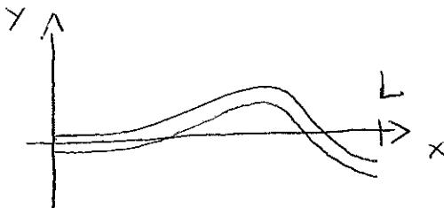
$$EI \frac{\partial^4 y}{\partial x^4} + m \frac{\partial^2 y}{\partial t^2} = p \leftarrow \text{last} \quad (=0 \text{ här})$$
