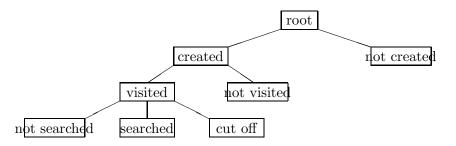
**Branching priority:** indicates whether the subsequent nodes in the tree are to be created simultaneously or not, and the order in which they are created.
