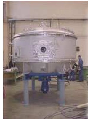
Figure 4: Ether products with different sizes can be dried in the vacuum dryer.
