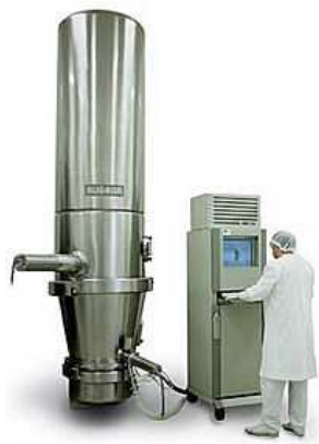
Figure 3: The fluidized bed requires that the cellulose ether must be ground to uniform particle size.
