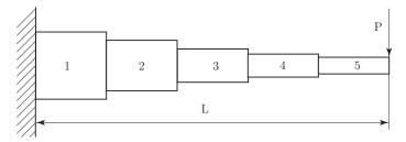
Figure 1: Stepped cantilever beam
