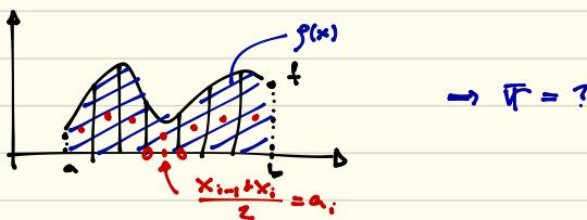
$$dm = f(a_i) \cdot f(a_i) \cdot dx \quad \text{and} \quad m = \int_a^b f(x) f(x) dx$$
