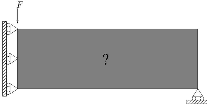
Figure 40: A cantilever beam: Initial solution,  $x_e = 0.5$  for all elements
