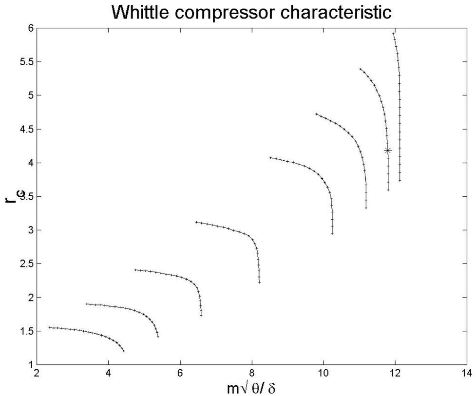
Figure 2: Whittle engine Compressor characteristic.
