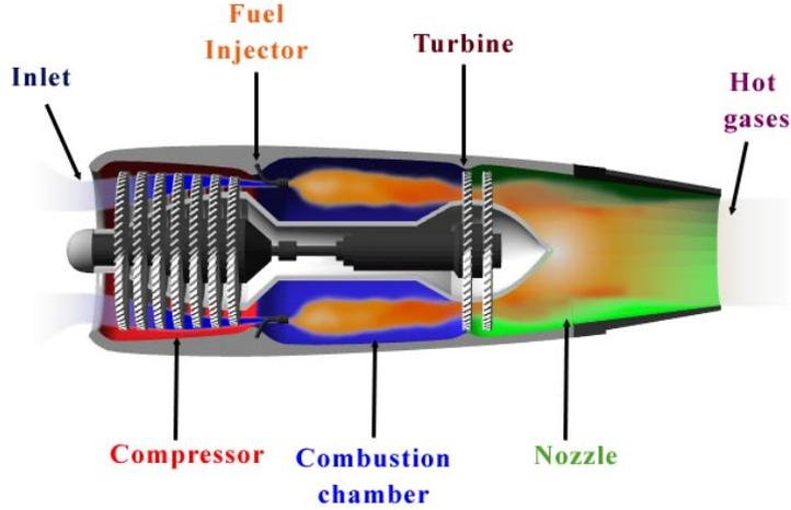
Figure 1: Turbojet engine components.
