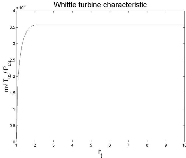
Figure 3: Turbine characteristic.
