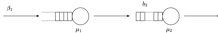
Figure 2.2. This simple network (tandem queue) illustrates how blocking of customers can occur when a station has a finite waiting space.
