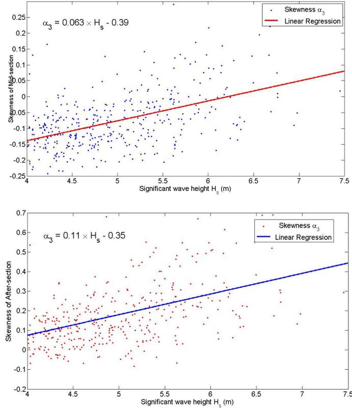
**Fig. 1:** Linear Regression of Skewness as a function of significant wave heights. Upper plot: Results for After-section; Lower plot: Results for Mid-section.
