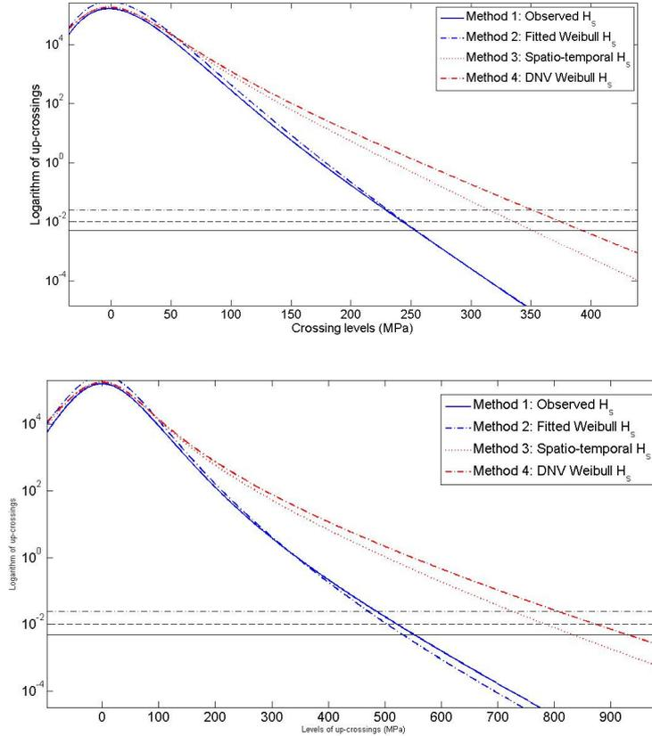
**Fig. 10:** Expected number of up-crossings and prediction of T-year extreme stresses  $x_T$ , computed by Winterstein's transform Gaussian approach on the basis of non-linear numerical analysis. Methods here represented are defined in Fig. 7. Upper plot: Results for After-section; Lower plot: Results for Mid-section.
