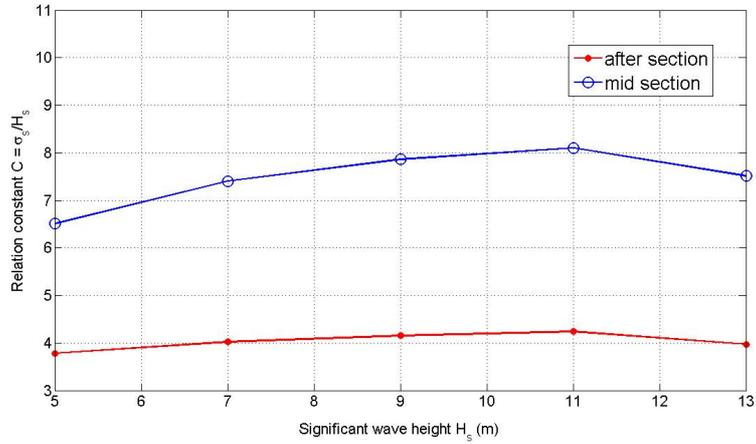
**Fig. 9:** Relation between standard deviation and significant wave height  $C = \sigma_x / H_s$  for both after section and mid section, by means of non-linear numerical analysis.
