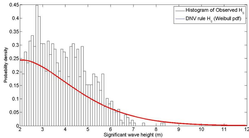
**Fig.6:** Empirical distribution of  $H_s$  measured by onboard radar, and long term distribution of  $H_s$  from DNV Rule.
