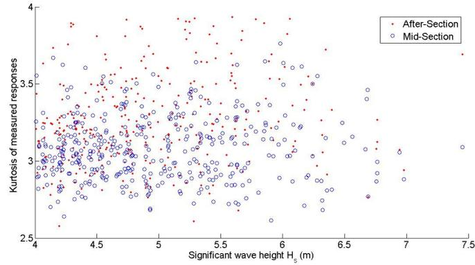
**Fig. 2:** Kurtosis of measured responses for both mid-section and after-section.
