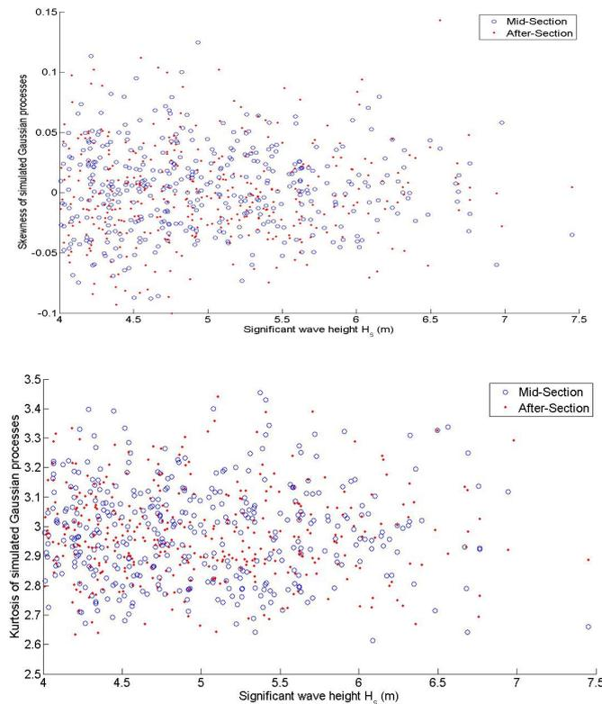
**Fig. 3:** Skewness (Upper) kurtosis (Lower) estimated from 30 minutes Gaussian responses with power spectrum estimated from the measured stresses for both mid-section and after-section.
