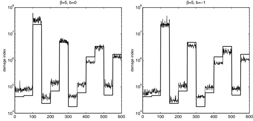
Figure 5: Six hundred simulated damage indexes with damage exponent  $\beta = 5$ , the irregular line. The corresponding observed damage indexes, the solid line. *Left*: LMA with symmetrical kernels  $b = 0$ . *Right*: LMA with asymmetrical kernels  $b = -1$ .
