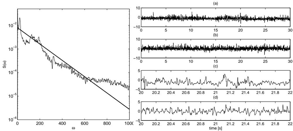
Figure 3: *Left*: Logarithms of empirical psd of  $F_z(t)$  (irregular line) and fitted exponential psd (solid line). *Right*: Plot (a) - one minute of measured force on a cultivator frame. Plot (b) - one minute of simulated LMA model of the force. Plot (c) - zoomed plot (a). Plot (d) zoomed plot (b).
