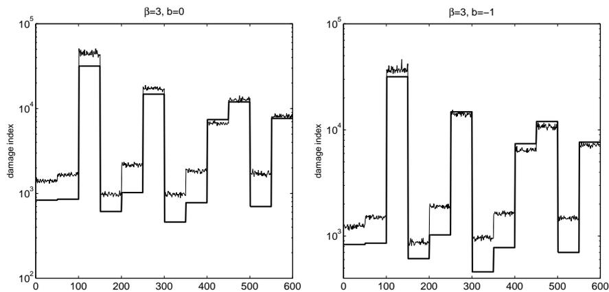
Figure 4: Six hundred simulated damage indexes with damage exponent  $\beta = 3$ , the irregular line. The corresponding observed damage indexes, the solid line. *Left*: LMA with symmetrical kernels  $b = 0$ . *Right*: LMA with asymmetrical kernels  $b = -1$ .
