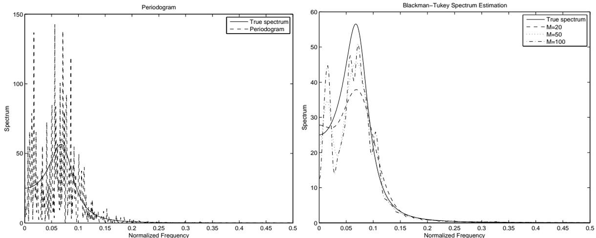
Figure 5: Examples of non-parametric spectrum estimation using the Periodogram (left plot) and the Blackman-Tukey method (right plot). The true spectrum is an AR(2) process.
