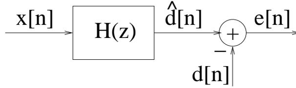
Figure 7: Optimal linear filter for signal estimation.
