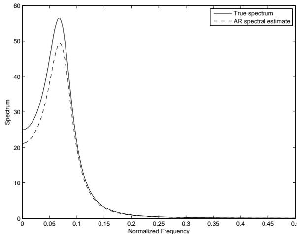
Figure 6: *Parametric AR spectral estimation using the YW method. Both the estimated and the true spectrum is an AR(2) model.*
