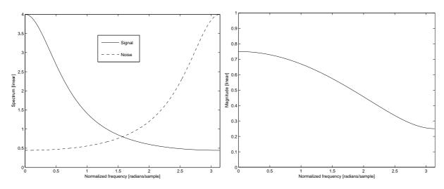
Figure 10: Signal and noise spectra (left plot), and magnitude of the corresponding length p = 2 FIR Wiener filter (right plot).
