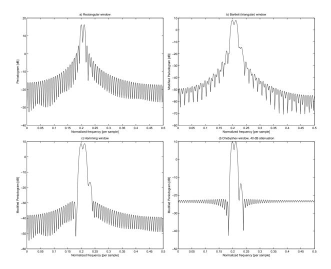
Figure 6: Spectral estimates for three sinusoids of frequencies  $f \in \{0.20, 0.21, 0.2295\}$ . The location of the f = 0.2295 component is at a sidelobe of the other components, and since its amplitude is 26 dB below the others it is completely masked by the strong neighbors when no windowing is used. The data windows are: a) Rectangular (no windowing), b) Bartlett (triangular), c) Hamming, and d) Chebyshev with 40 dB attenuation. The number of samples is N = 128.
