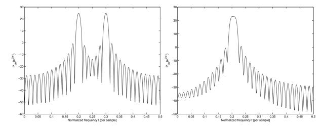
Figure 5: Periodogram for two sinusoids of frequencies  $f_1 = 0.2$ ,  $f_2 = 0.3$  (left plot), and  $f_1 = 0.2$ ,  $f_2 = 0.21$  (right plot). The number of samples is N = 64, so the frequency resolution is  $\Delta f = 1/N = 0.0156$ . In the right plot,  $f_2 - f_1 = 0.01 < \Delta f$ , and the frequencies cannot be resolved.
