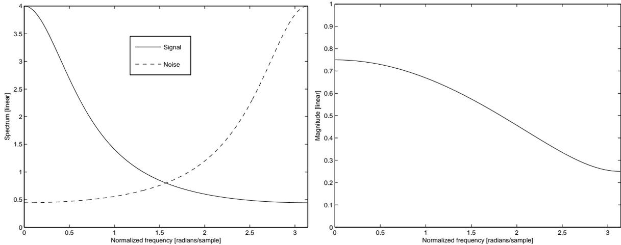
Figure 10: *Signal and noise spectra (left plot), and magnitude of the corresponding length  $p = 2$  FIR Wiener filter (right plot).*
