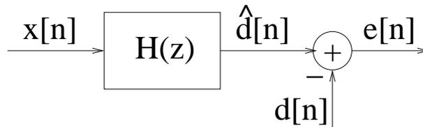
Figure 9: Optimal linear filter for signal estimation.
