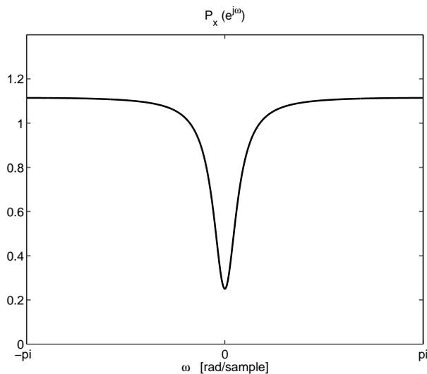
Figure 2: The power spectral density of the ARMA(1,1) process  $x[n]$ .
