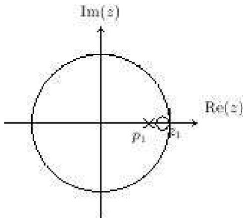
Figure 1: An illustration of the pole  $p_1$  marked with a cross and the zero  $z_1$  marked with a circle for  $H(z)$ , i.e., the so called pole-zero plot for  $H(z)$ .
