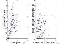
Wave data from North Sea. Scatter plot of crest period and crest amplitude (left); crest period  $T_c$  and crest amplitude  $A_c$ , resampled from original data (right).
