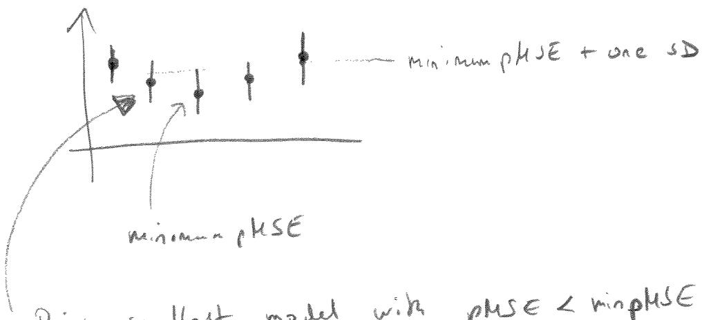
Pick smallest model with  $pMSE < \text{minpMSE} + SD$
