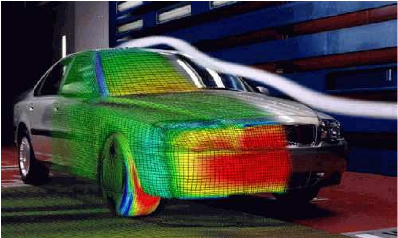
Numerical solution of the Navier-Stokes equations.
