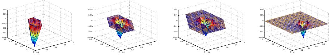
Figure 1: A typical localized solution  $U_{f,i}$  of the fine scale equations in a smooth region using one, two, three layer stars, and the entire domain.
