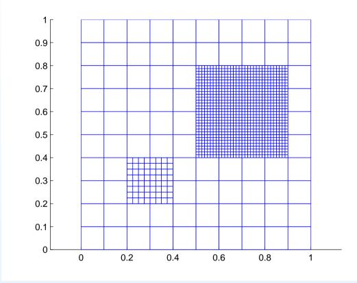
We let H be coarse scale mesh size and h be fine scale mesh size. Further we let L denote the number of layers of coarse elements in the patch. Typically homogeneous Dirichlet boundary condition are used.
