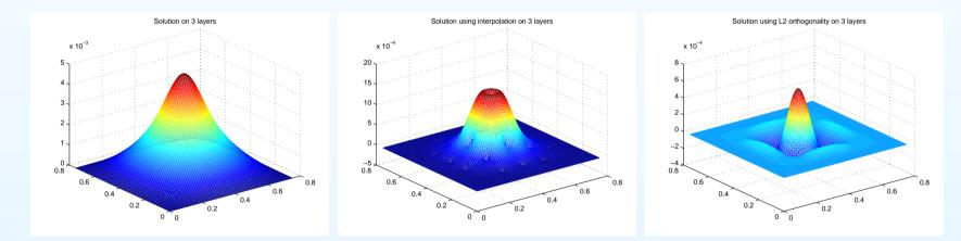
To the left  $\mathcal{W} = \mathcal{V}_c \oplus \mathcal{V}_f$ , middle  $\mathcal{W} = \mathcal{V}_f$  using hierarchical split, and right  $\mathcal{W} = \mathcal{V}_f$  using  $L^2$ -orthogonal split.
