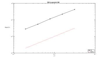
Illustration of the strong error of Euler-Maruyama's scheme for the geometric Brownian motion
