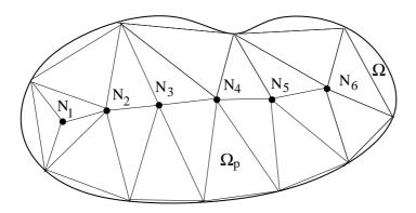
Here we have 6 internal nodes  $N_i$ ,  $1 \le i \le 6$ .  $\Omega_p$  is the *polygonal* domain inside  $\Omega$ , which is triangulated.
