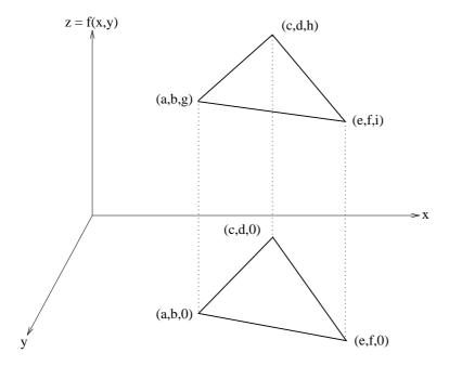
This figure illustrates how piecewise linear function on a triangle is determined by its values at the vertices of the triangle.
