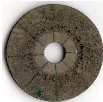
corroded Mg plate
