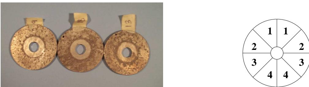
Figure 1: Left: Specimens of magnesium plates. Right: Numbering of the sectors in terms of their location.
