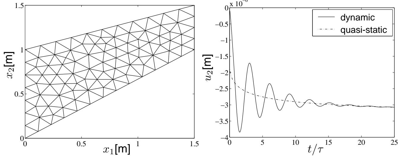
$$u(x, 0) = 0 \text{ m}, \quad \dot{u}(x, 0) = 0 \text{ m/s}, \quad f(x, t) = 0 \text{ N/m}^3,$$
