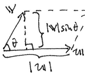
$$\begin{aligned} \text{Area parallelogram} &= \\ &= |u||v| \sin \theta = |u \times v| \end{aligned}$$
