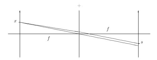
In the geometrical optics approximation, rays from a point x in one focal plane is refracted to parallel rays by the lens, and the ray through the center is not refracted. This implies that a ray from the point x to the point s has travel length
