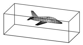
Discretize (divide into small volume elements) the air in the box and outside the aircraft. Mesh generation (using m3d, an ITM-project, Swedish Institute of Applied Mathematics) on one RS6000 processor:
