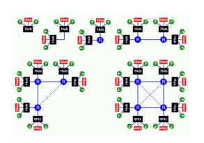
More than two nodes are connected via a router. A router has six ports. Hypercube configuration. When the system grows, add communication hardware for scalability.
