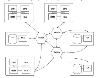
Switches forward packets between two of their ports based on an established routing table and the addressing information stored on the packets. A subnet, like the one above, can be connected to another subnet by a router.
