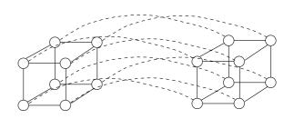
A 4-dimensional hypercube. Generally, a hypercube of dimension d+1 is constructed by connecting corresponding processors in two hypercubes of dimension d.
