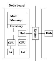
The hub manages each processor's access to memory (both local and remote) and I/O. Local memory accesses can be done independently of each other. Accessing remote memory is more complicated and takes more time.
