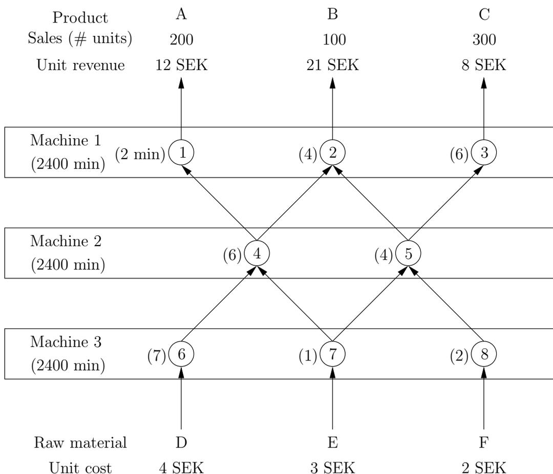
Figure 1: The production process.
