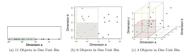
Figure 1: The *curse of dimensionality*. Data in only one dimension is relatively tightly packed. Adding a dimension stretches the points across that dimension, pushing them further apart. Additional dimensions spreads the data even further making high dimensional data extremely sparse.
