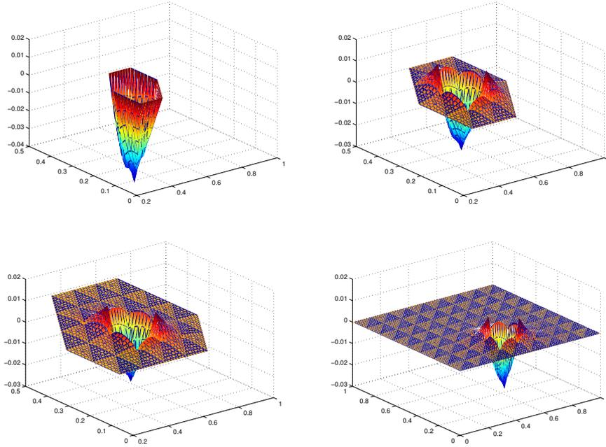
Figure 1: A typical localized solution  $U_{f,i}$  of the fine scale equations in a smooth region using one, two, three layer stars, and the entire domain.
