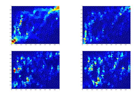
Figure 8: Relative error in energy norm: 106%, 16%, 10%, and 8%.
