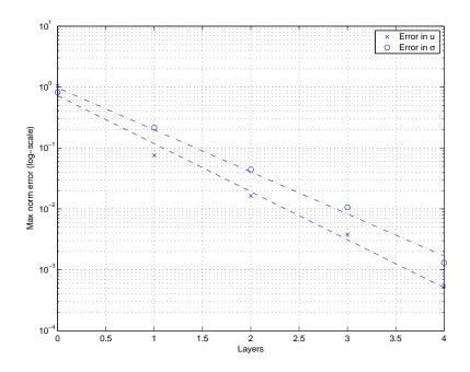
Figure 5: Max norm error (compared to reference solution) in log scale versus number of layers.
