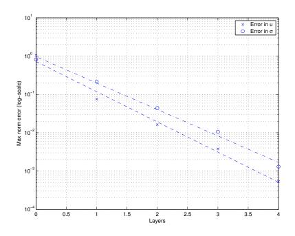
Figure 5: Max norm error (compared to reference solution) in log scale versus number of layers.
