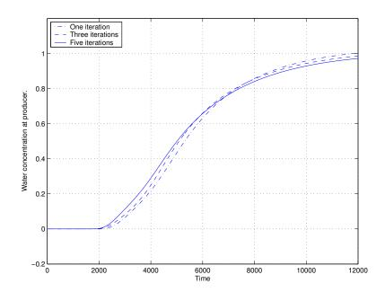
Figure 15: The water concentration at the producer at different times for approximations after one, three, and five iterations.
