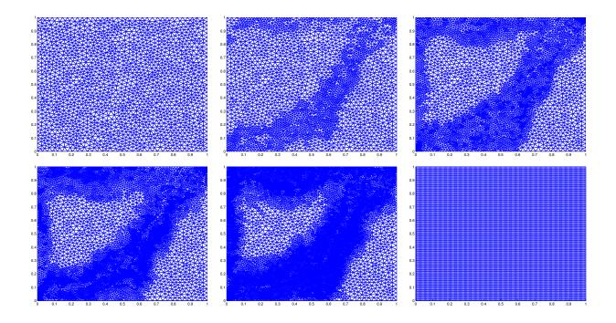
Figure 13: Mesh after each of the five iterations. Rectangular mesh for the flow problem.
