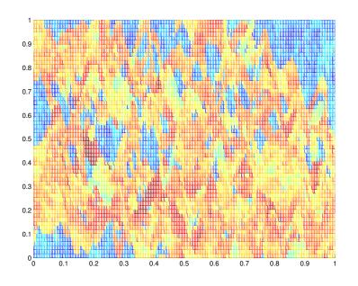
Figure 3: 2D slice of the permeability a (in log scale) taken from the tenth SPE comparative solution project.
