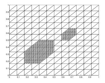
To the right we see a mesh star to the left what we call a two layer mesh star. The coarse mesh size is denoted H and the fine mesh size is denoted h.
