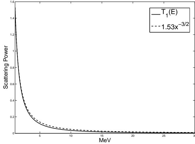
FIGURE 1. Scattering power for elastic scattering
