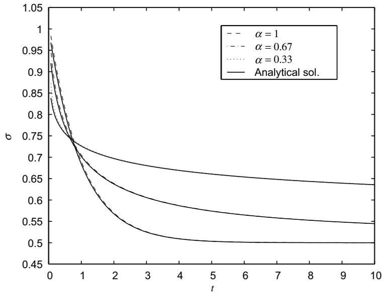
Fig. 2. The stress response due to a unit step strain imposed at time  $t = 0$ . Numerical solutions are compared with analytical solutions for different values of  $\alpha$ .
