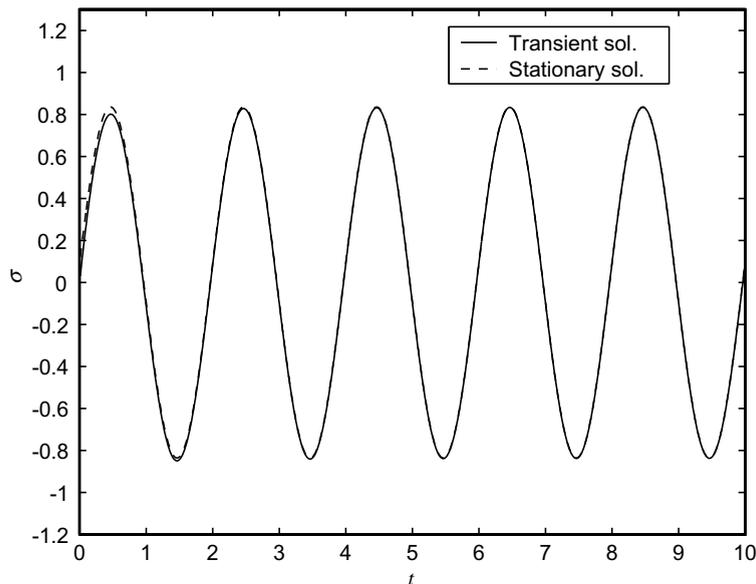
Fig. 3. The stress response due to the harmonic strain in (7.2) using sparse quadrature. For comparison the stationary solution is also shown.
